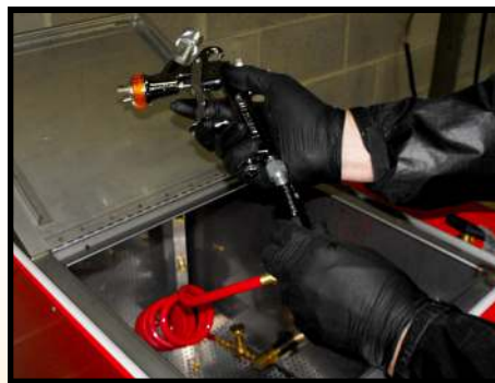
POWERCLEAN™ .... Supply's Compressed Air to the Spray Gun During the Cleaning Process, Protecting the Air Passageways
