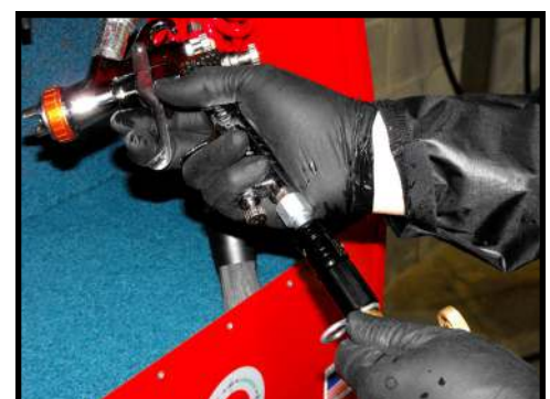
POWERCLEAN™ .... Supply's Compressed Air to the Spray Gun During the Cleaning Process, Protecting the Air Passageways
