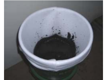
Paint Waste collected by the Filter
